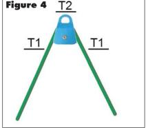
to the pulley in Figure 4, the values still must balance. In Figure 4, both numbers where the rope enters/exits the pulley must be the same to balance the T's crossbar, and the number near the eye of the pulley must equal their sum to keep the T's stem in balance with the crossbar.
