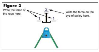
It is helpful to think of the T's crossbar as a balance-beam scale. The values on the left and right sides of the crossbar must be the same so the crossbar is balanced. Similarly, the value on the end of the T's stem must equal the sum of the two values on the crossbar. This is an important principle of the T-System—the T must balance from both left to right and top to bottom.
