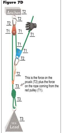
the value at the eye of the pulley will always be T2. This has been the case in these examples, but it will not always be the case.
